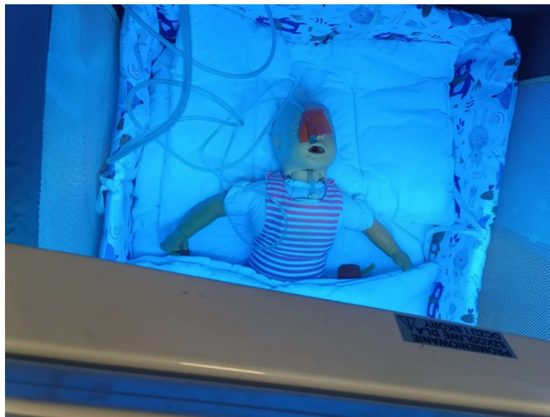
Figure 1. UV lamp analysis - identification of CO 2 location in the crib volume.
